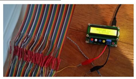
8/ Add a 300pf capacitor (I glued the wires and used Velcro to bond the capacitor)
