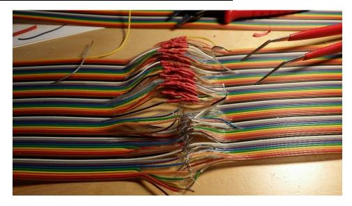
4/ Continue to solder wires and do not forget to make one loop alone to allow coupling
