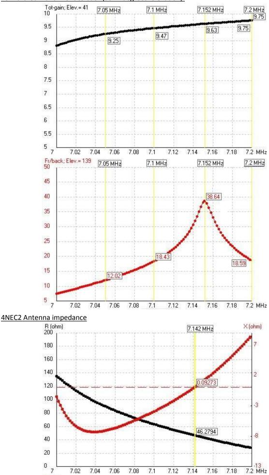
Forward Gain and Front to back (at 41 degrees' elevation).
