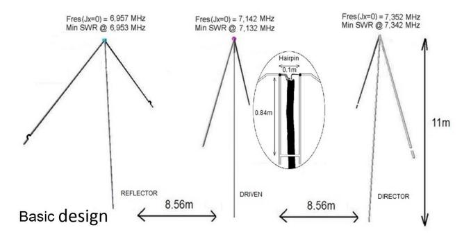
6/ The installation of the parasitic elements on the fiberglass mast is illustrated below:
